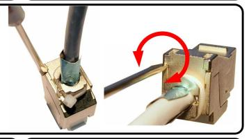
KJS458TL-series keystone jacks can be connected directly to telecommunications bonding/grounding system using compliant grounding conductor equipped with 2.8 x 0.5-mm (0.110 x 0.020-in) female disconnect and grounding post 1 located on fixed part of grounding clip.
