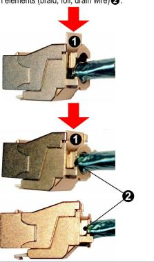
Thread plastic cable tie 1 through opening on fixed part of grounding clip 2, wrap it around both clip parts and tighten slightly.
